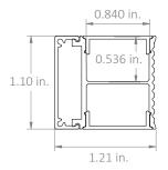
$\label{eq:charge} Chromapath^{\texttt{B}} \ \text{Bundle: SCONCE Channel is compatible with custom cut and soldered} \\ DOUBLE \ \text{BLAZE}^{\texttt{M}} \ \text{LED Tape Light } \textbf{only}.$
